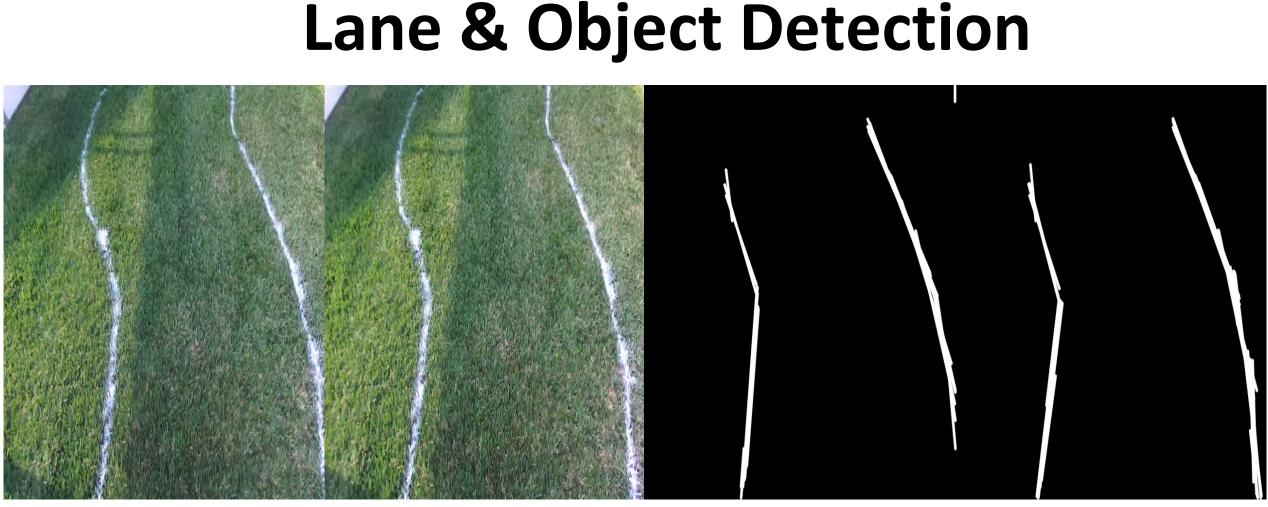
Filtering – Utilizes a Convolutional Neural Network (CNN) to perform semantic segmentation to identify lanes. **Thresholding –** Used to remove noise produced by the CNN and remove entities the algorithm poorly differentiates such as shadows.
